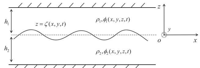
FIG. 1. The physical sketch of the two-fluid system with related notations.
