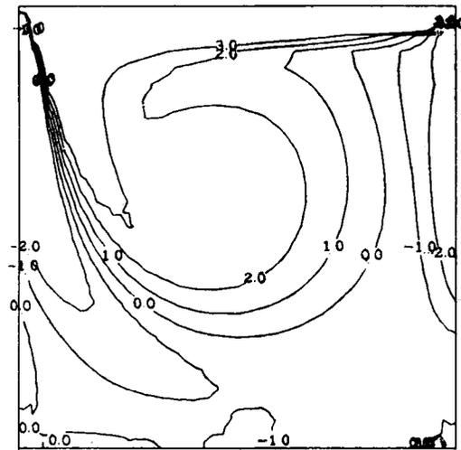
Figure 7. Contour of vorticity  $\omega$  in the case  $Re=400$
